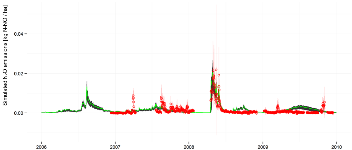
Figure 23 Simulated N 2 O emissions [kg N-N 2 O / ha] including the uncertainty bands resulting from the BC. Green line: median, black lines: 25 and 75 percentile, grey area: estimated uncertainty range, red circles: field measurements and measurement errors
