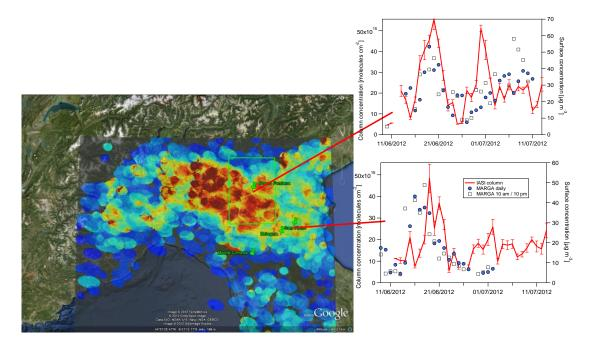
Figure 5. Composite image of the NH<sub>3</sub> column concentration field derived from IASI by ULB for the measurement campaign. Also shown are the daily time-series averaged over the area (green box) centred around Bosco Fontana and San Pietro Capofiume (red lines), compared with groundobservations by MARGA/GRAEGOR (operated by NERC/ECN), comparing full-day averages (blue symbols) and measurements that coincide with the 10:30 am satellite pass over (empty symbols).
