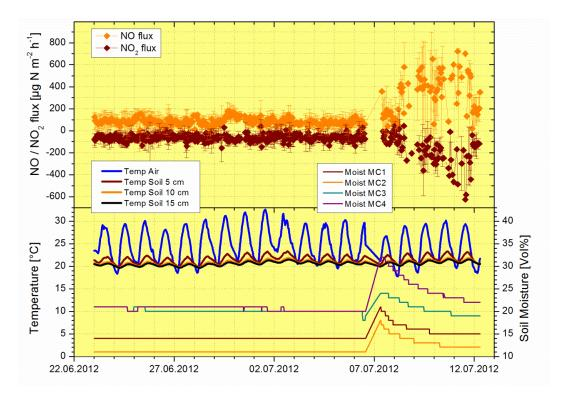
**Figure 4.** Dynamics of NO and NO<sub>2</sub> flux ( $\pm$  SD) at the soil-atmosphere interface, air and soil temperature across soil profile and volumetric soil water content (0-8 cm) for the period June 22<sup>nd</sup> to July 12<sup>th</sup> 2013 at Bosco Fontana Forest site. The increase in the fluxes is related to a precipitation event on 7-July.
