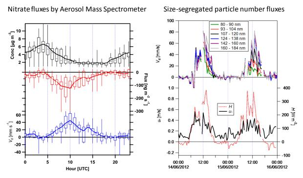
**Figure 3.** (a) Average diurnal cycles of the concentrations, flux and deposition velocity of aerosol nitrate as measured by the Aerosol Mass Spectrometer flux system operated by NERC. (b) Example time-series of the size segregated deposition velocity derived from particle number fluxes with an optical particle spectrometer (NERC, UGOT), in relation to heat flux (H) and friction velocity ( $u_*$ ).
